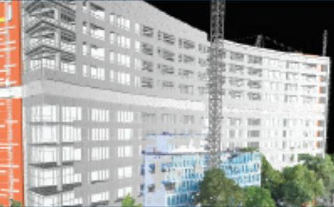
BIM, or Building Information Modeling, is a sophisticated process for creating and managing all of the information on a project—before, during and after construction. BIM enables the design team, constructor and owner to work together with a 3D generated model resulting in better design coordination and improved constructability. Once the building is completed, BIM delivers a complete set of information, allowing the owner to efficiently manage and maintain the building.
